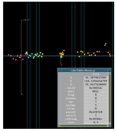
Simulated Hijing event in STAR showing reconstructed points and results of tracking. A cut plane is used to eliminate the far half of the barrel and make the images more understandable.
