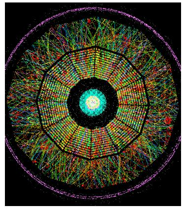
Reconstructed laser tracks in STAR. The view is along a track. The image is magnified and the z-axis is expanded enabling a resolution of approximately 100 microns and 20 micro-radians. You can get the actual point data by picking it.
