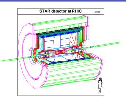
The STAR experiment has been assembled at the Relativistic Heavy Ion Collider (RHIC) at the Brookhaven National Laboratory to investigate high-energy collisions of heavy nuclei. The ultimate goal is the discovery of the phase transition to a quark-gluon plasma.
