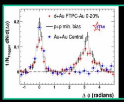
RHIC AA + pp + dAu results: Hard-scatterings are initially present; Suppression phenomena in central Au+Au are due to final-state interactions. (consistent with jet quenching)
