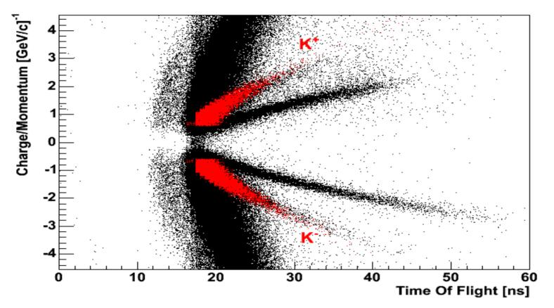
Standard Identification via Time Of Flight from the EMC and Momentum determined by Track Curvature in Magnetic Field
