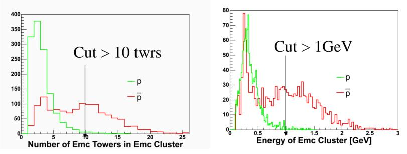
As expected the main difference is the deposited energy and the Number of towers which make up this cluster. Cut at 10 towers and 1 GeV Cluster Energy.
